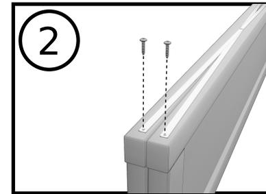
Line up the holes in the cross brace with the marks and screw directly into the upright.
